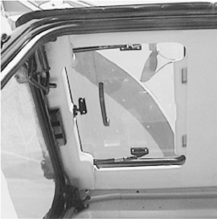
Cat 320B Skylight
