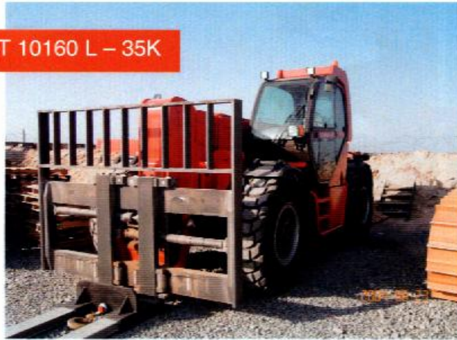
Hydraulic Forkpositioner with side shift Forks together - backrest
