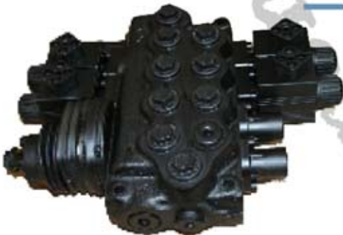
SINGLE-BODY DISTRIBUTOR WITH 4 SERIAL VALVES
