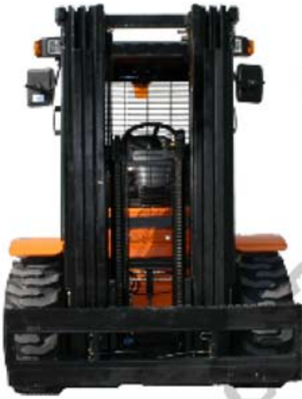
THREE-STAGE MAST WITH 4 CYLINDERS AND INTEGRATED SIDE SHIFTER FOR MAXIMUM VISIBILITY
