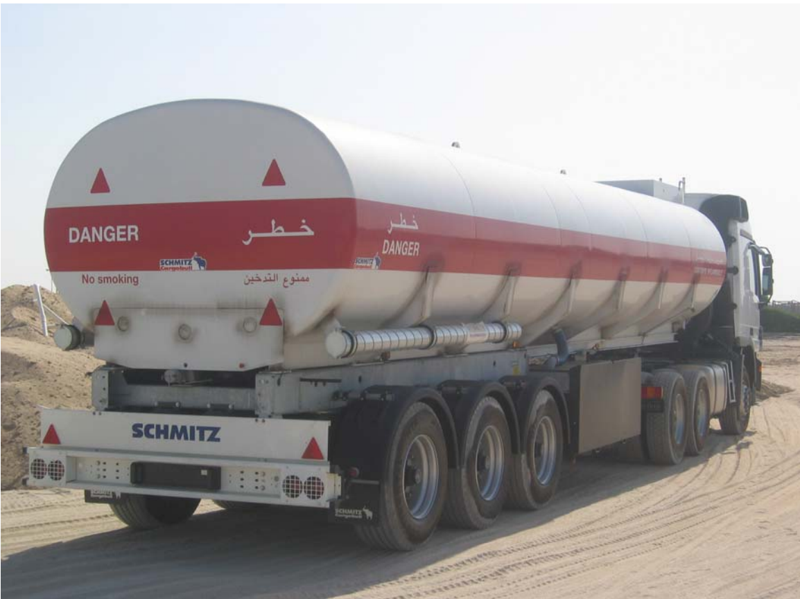
Schmitz Diesel Tank Semi-Trailer 10'000 US gallon, Type STA 27/L 10000-SK-D
