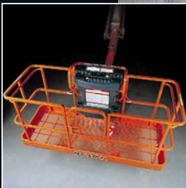
Large Operator Work Platform
